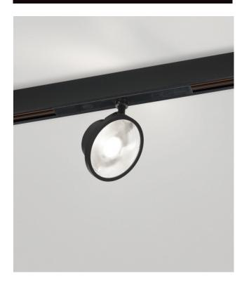
Designed around its flat optics, Haloscan combines ultra-minimalistic looks with a pleasurable light effect. The light is softly spread by the plane lens, creating up to 4 different beam angles, from spot to floodlight and even linear light. To smoothly turn and tilt, Haloscan uses the Ex-Centric Rotation System, an asymmetrical hinge that combines rotating and tilting abilities in one swift move.
